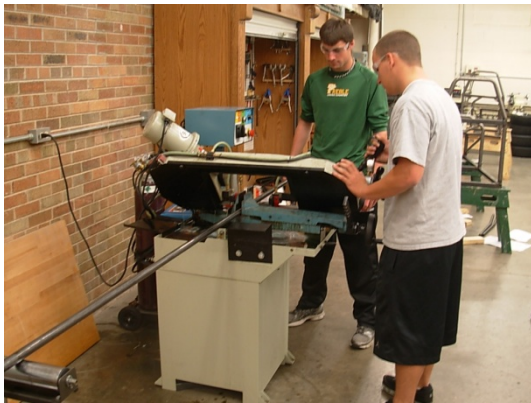
Devan and Matt cutting 1 1/2" tubing for a support brace on the front of the chassis.
